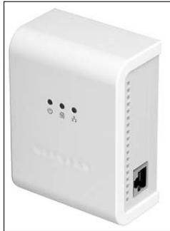
Figure 5-2: Netgear's wall- plugged Ethernet bridge.
