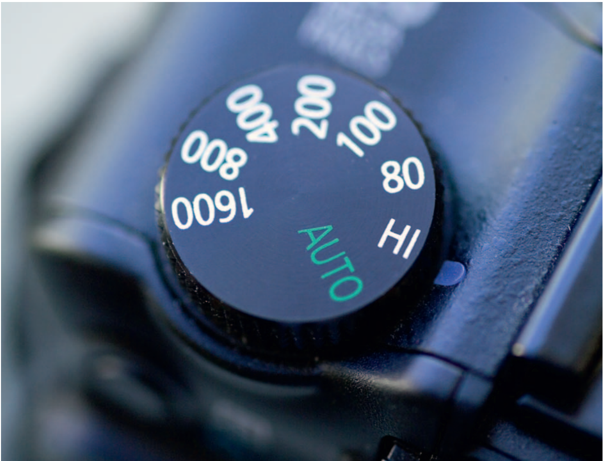
FIGURE 5.4 An ISO dial on a quality compact camera. Avoid Auto and Hi (high)! Stick to settings below 200 ISO. Not all cameras have a separate dial for ISO settings; some have ISO settings buried in a submenu. © Douglas Freer
