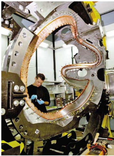
Surely hard. The reactor's coils look like something Salvador Dalí might have sculpted. Joining them proved hugely difficult and expensive.
